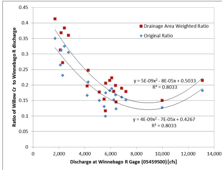
Figure 3. The ratio of area-weighted discharge at the upstream Willow Creek study boundary to discharge at the Winnebago River USGS gage (05459500) is plotted with respect to the historic discharge at the Winnebago River USGS gage (05459500)
