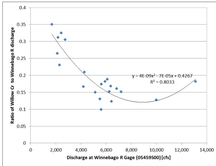
Figure 2. The ratio of discharge at the Willow Creek USGS gage (05460100) to discharge at the Winnebago River USGS gage (05459500) is plotted with respect to the historic discharge at the Winnebago River USGS gage (05459500)
