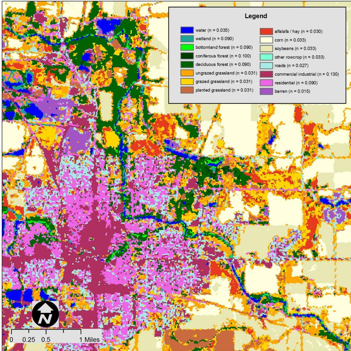
Figure 4. Manning’s roughness values assigned to corresponding the USGS 2001 National Land Cover Database classifications.
