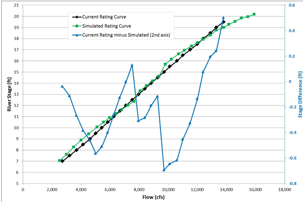
Figure 5. Plot comparing the established USGS rating curve compared to simulated rating curve at the river gaging station (05459500).
